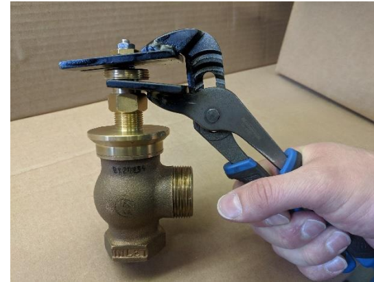
4- Install stainless steel nut and lock in place. Remove tool by pulling toward you.
